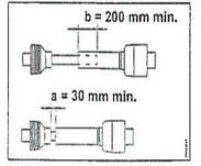
The P.T.O must be cut to a proper length, so it does not "bottom out" and bind. Remove the PTO to perform this operation. If the PTO is not cut to the proper length, it may cause damage to the PTO, gearboxes etc. See illustration for proper measurements.
